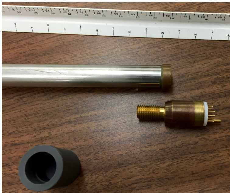
Figure 3—SHORTING PLUG BESIDE TOOL
