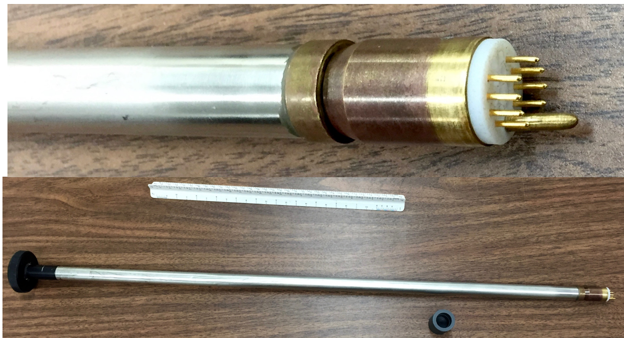
Figure 2- EXPANSION OF A SHORTING PLUG THAT MUST BE REMOVED FROM THE CRYOSTAT PRIOR TO DECOMMISSIONING.
