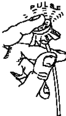
Using a dipstick as a helium level probe
