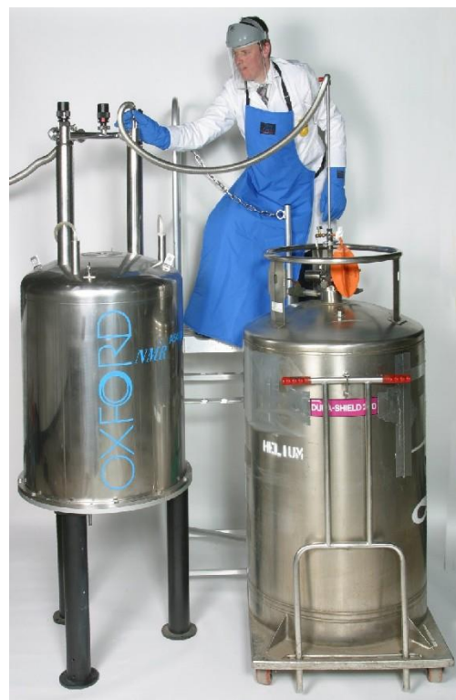
Figure 16 Inserting syphon leg into cryostat and making a gas tight seal
