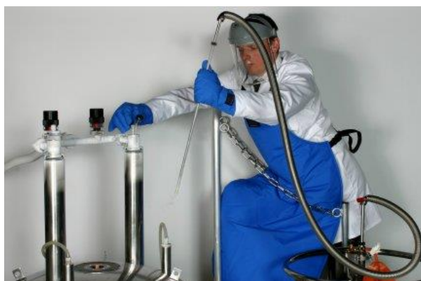
Figure 20 Syphon leg just after removal from cryostat
