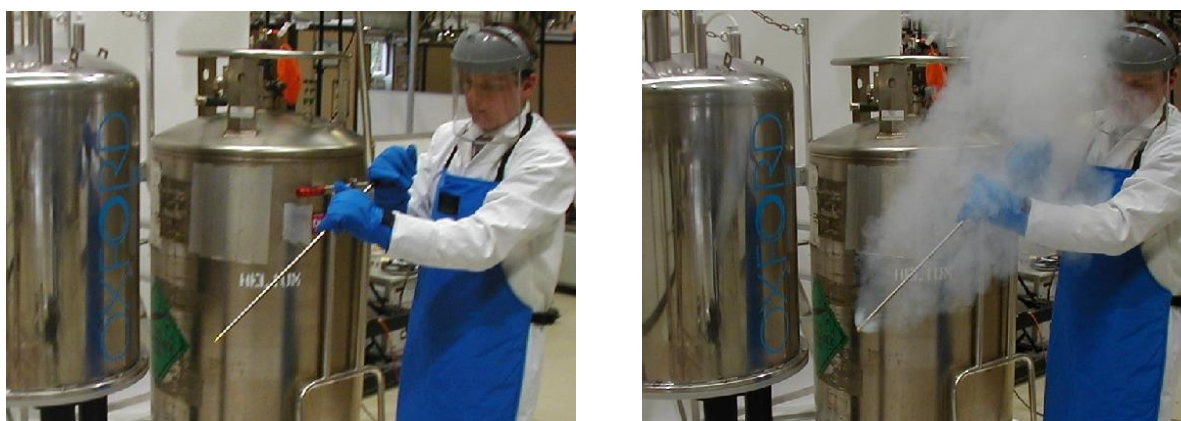
Figure 14 Pre-cooling the syphon
