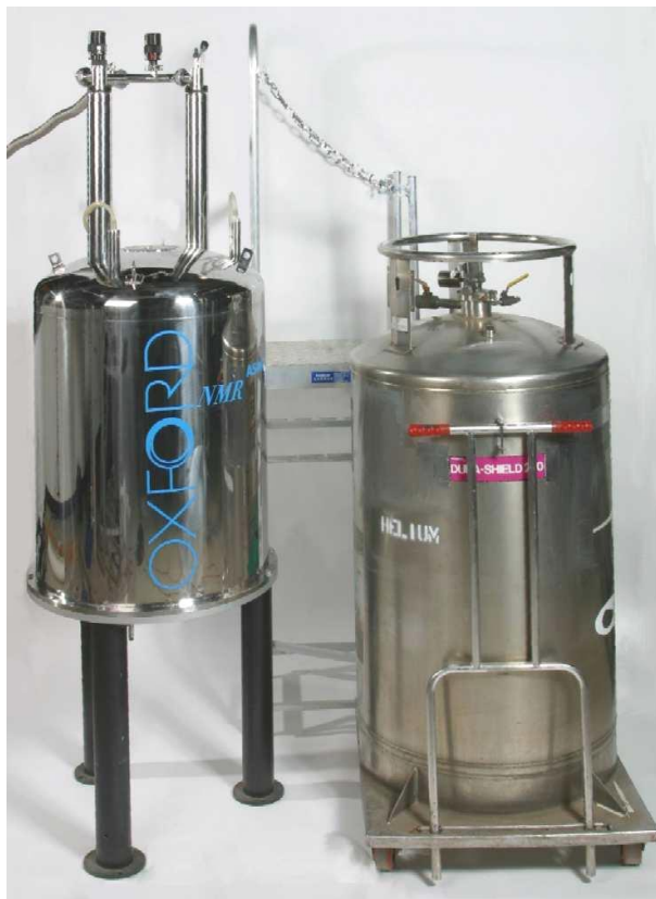
Figure 4 Main items for helium refill: cryostat, climbing platform and storage dewar
