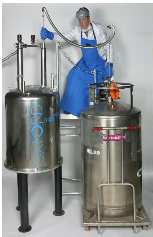
Figure 16 Inserting syphon leg into cryostat and making a gas tight seal
