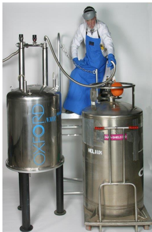
Figure 17 Full insertion of syphon leg into storage dewar
