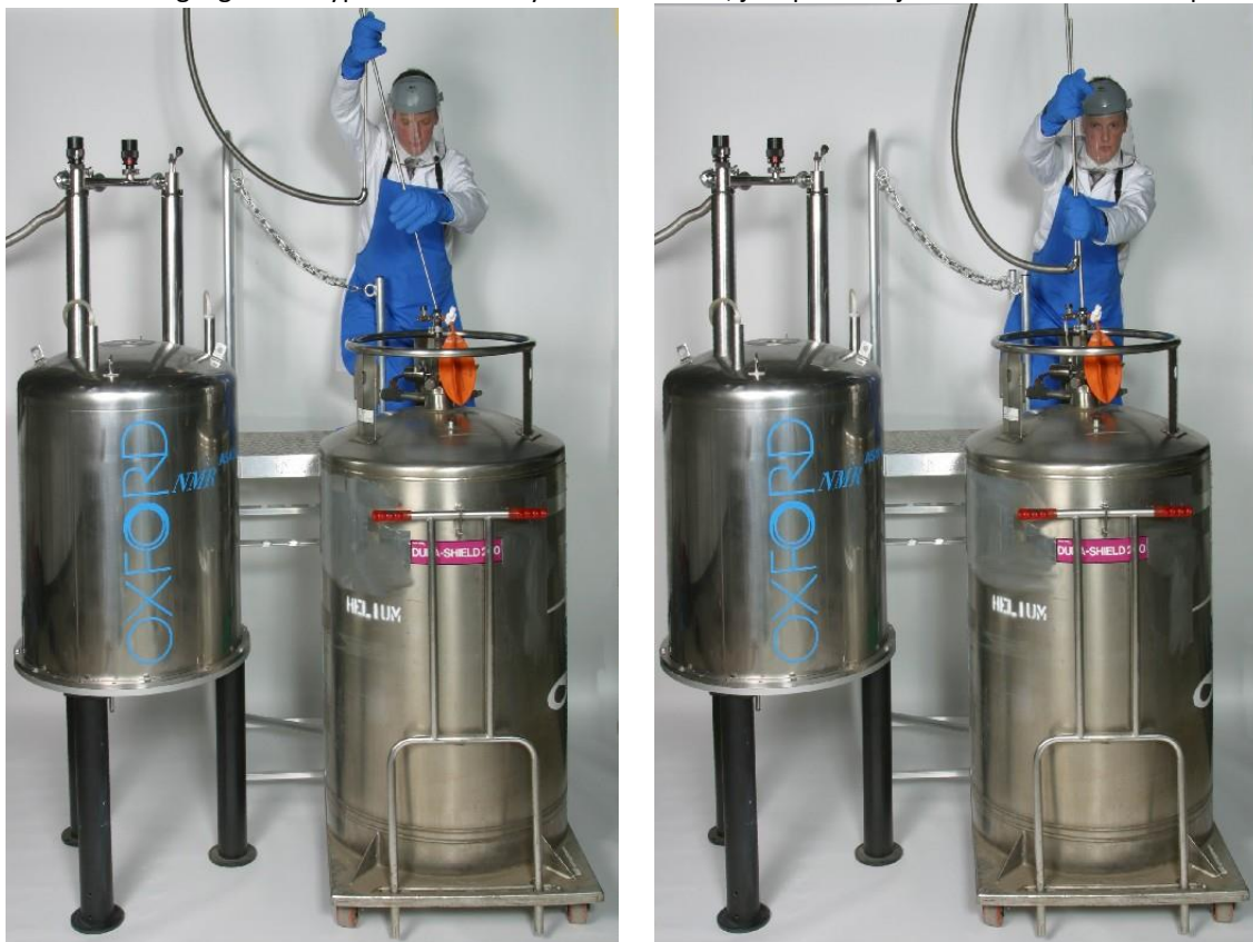
Figure 12 Inserting syphon leg into storage dewar
