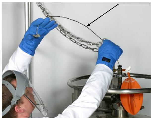
Figure 3 Using a dipstick to measure helium level
