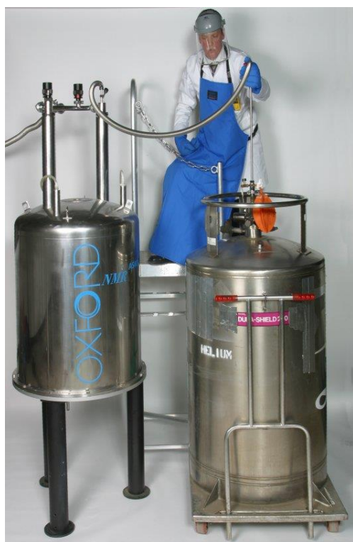
Figure 17 Full insertion of syphon leg into storage dewar
