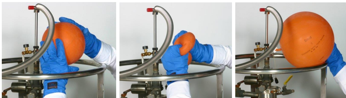
Figure 13 Sequence showing inflation of bladder
